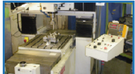
SIP HAUSER NO42 JIG BORER
